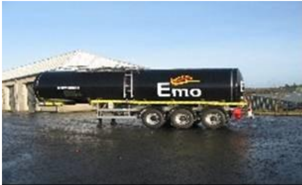
Image 41 Example of an ADR tank designed for the transportation of gas oil or black oil
