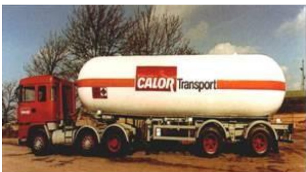
Image 43 Example of a pressure tank designed for carrying liquefied petroleum gas
