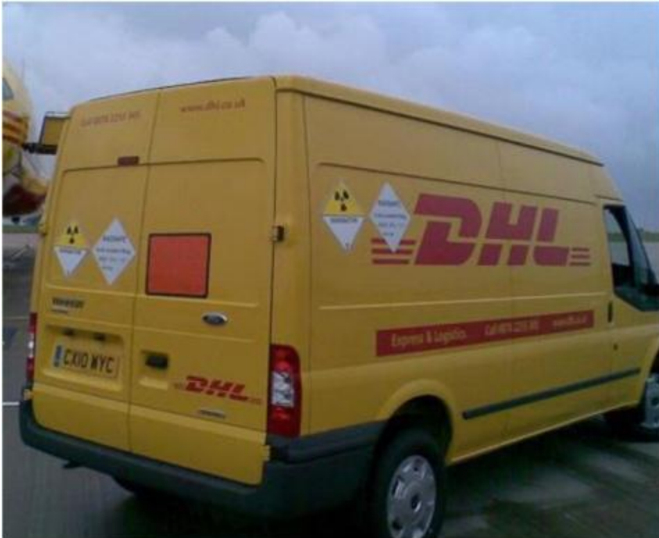
Image 14 Type of vehicle used by DHL to transport packaged dangerous goods in the UK. The class 7 and 'Radsafe' labels would be
