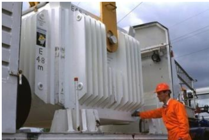
Image 31 Irradiated fuel transport flask being loaded onto a train
