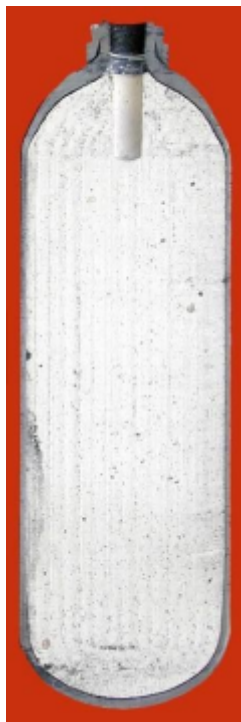
Image 89 Cross section through an acetylene cylinder showing the 'gas space'
