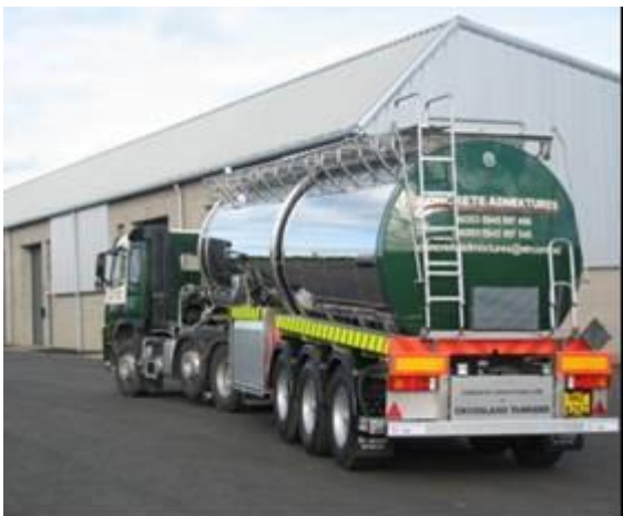
Image 40 Example of a non-pressure, stainless steel, multi-compartment tanker
