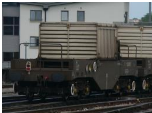
Image 110 Fuel flask used to transport spent fuel back to Sellafield
