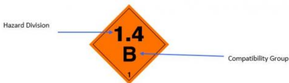
Figure 2: Transportation hazard warning diamond for UN Hazard Division 1.4 to 1.6 and Compatibility Group (N.B. No 'bomb burst')
