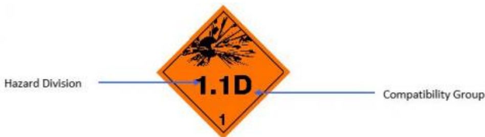
Figure 1: Transportation hazard warning diamond for UN Hazard Division 1.1 to 1.3 and Compatibility Group
